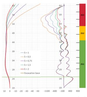
Horizontal displacement (mm) Bending moments envelope (kNm)
