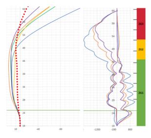
Horizontal displacement (mm) Bending moments envelope (kNm)
