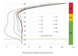
Figure 6 – Displacements after each excavation level
