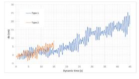
Figure 10 - Differential horizontal displacements: type 1 seismic activity (blue); type 2 seismic activity (orange)
