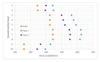
Figure 12 – Anchors axial loads: static conditions (blue); type 1 seismic activity (orange); type 2 seismic activity (purple)
